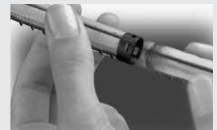
Step 3: Combine screen tubes to desired length.
