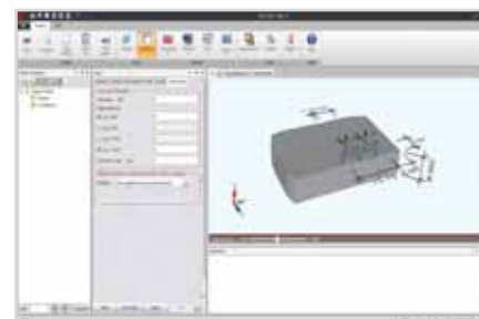
Screenshot 2: Input GUI (Graphic User Interface), HALFEN HTA Software
